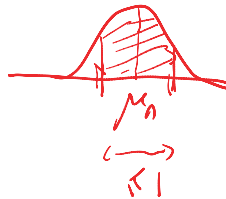
Figure 1: Gaussian posterior centered on \mu_n . The shaded interval contains 95% probability mass and has width 1.
