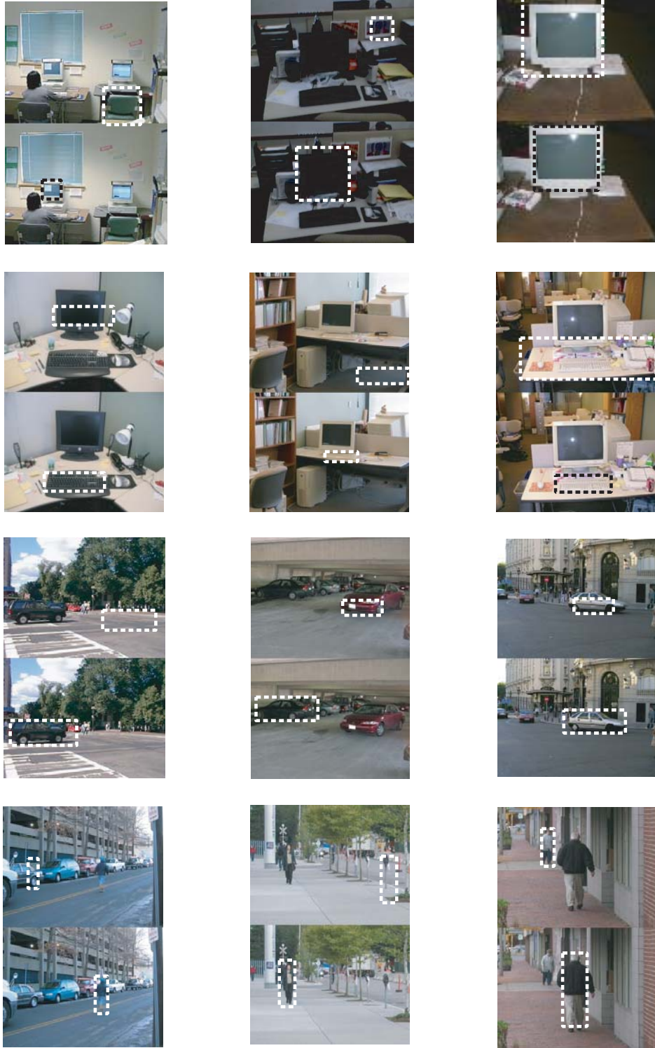
Fig. 11. Examples of localization of screens, keyboards, cars and pedestrians. Within each image pair, the top image shows the most likely location/scale of the object given local features ( \arg \max P(X|L) ), and the bottom image shows the most likely location/scale of the object given local and global features ( \arg \max P(X|L, G) ).
