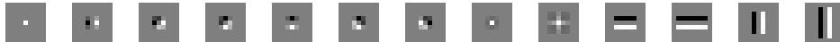
Fig. 2. The bank of 13 filters. From left to right, they are: a delta function, 6 oriented Gaussian derivatives, a Laplace of Gaussian, a corner detector, and 4 bar detectors.
