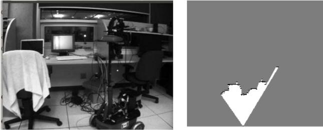
Figure 2: Camera image (left), Occupancy map representing bird's-eye view of obstacles (right)
