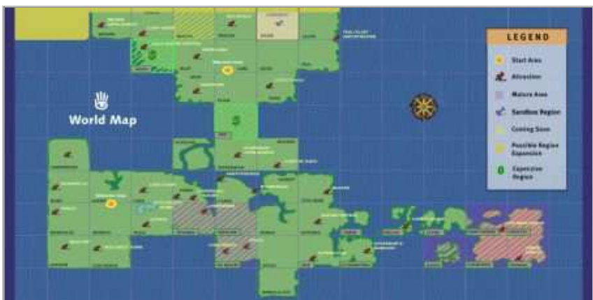
Map of the Second Life world. It's also a diagram of our scalable server grid. Each square on the map represents 16 virtual acres of land in Second Life. Each square also represents one "sim" - an off-the-shelf Linux server edge-connected to up to four neighboring servers. More land is added by adding more "sims".
