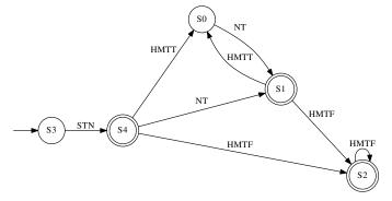
Fig. 3: StringTokenizer's SpecForge Model. "STN": StringTokenizer(). "HMTT": hasMoreTokens() = true. "HMTF": hasMoreTokens() = false. "NT": nextToken().
