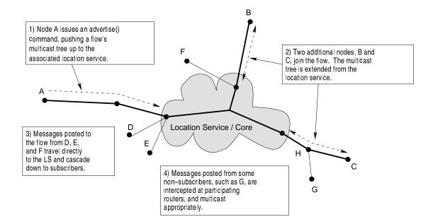
Figure 3.4: Multicast routing with flows
