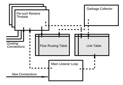
Figure 4.1: Structure of the Flow Router
