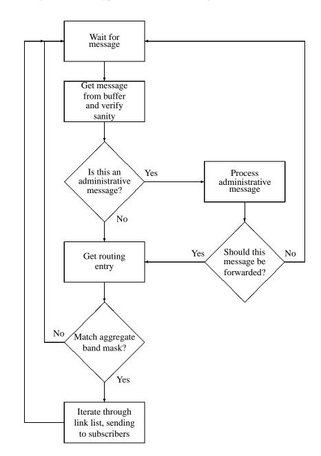
Figure 4.2: Prototype Flow Router – Routing Mechanism
