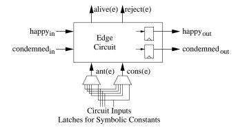
**Figure 2: Sub-Circuit for Each Edge.** Each edge corresponds to a sub-circuit that receives incoming tokens for happy and condemned paths, updates the tokens depending on whether the current antecedent and consequent pass, and passes the tokens onward on the next clock cycle.
